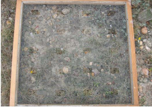
**Figure 2.** A planting grid (50 cm x 50 cm) comprising hardware cloth (wire mesh) within a wooden frame, with 20 planting rectangles (3.2 cm x 4.5 cm) cut into the mesh.
