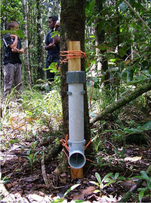
Figure 2. Front view of a 'hockey stick' dispenser designed for 20 g fixed bait blocks. Note the vertical wire at the entrance to prevent large Achatina snails from raiding the bait blocks. The dispenser is raised 10 cm above ground to deter snails and tenrecs and also to reduce humidity from the ground.
