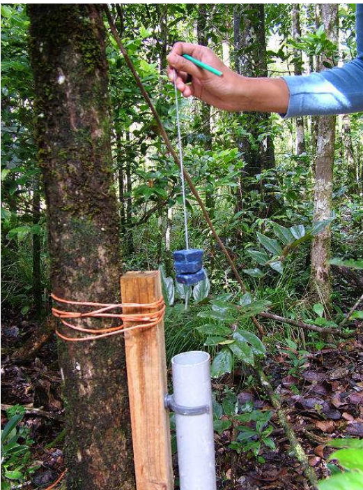
Figure 3. The 20 g wax blocks are threaded onto a length of thick wire. Checking the bait and refilling is straightforward.
