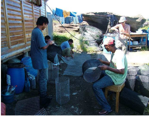
Figure 1. MWF staff making plant cages in preparation for the planting season. The wire is purchased in rolls, cut to size, rolled into shape and covered with shade cloth.
